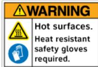
*Burn Hazard -- Hot Surface.* Outer surface temperatures of the Cleanstream 550/H1500 may reach 120 °C during normal operation.
